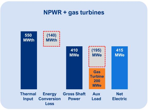
Integrating simple cycle gas turbines with Net Power doubles power output with half of the emissions of a standard 200MWe gas plant
